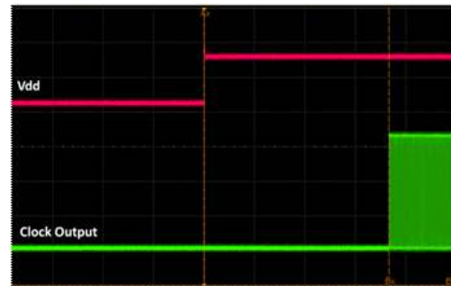
Figure 16. Startup Waveform vs. Vdd
