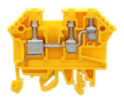
Feed-through terminal, Screw connection, Mounting type:Mounting rail TS 35/7.5 and TS 32, Rated cross-section: 4 mm², Width: 6 mm, Colour: Yellow
