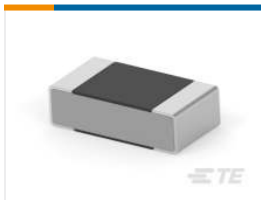
TE Part #8-1879135-6 RN 0603 9R09 0.1% 10PPM 5K RL
