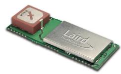
The Laird Embedded Bluetooth® Module is specifically designed for applications that demand a robust and reliable Bluetooth connection. This product is designed with solder connections that allow the module to be mounted directly into your own designs and potted or enclosed within metal housing while exposing a high performance multilayer ceramic antenna.
