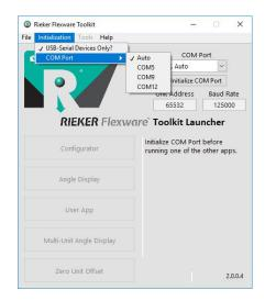
To access and configure the Flex inclinometer, install the Flexware<sup>TM</sup> Toolkit App, which is provided on the included USB Flash Drive. Connect the USB Interface Cable to the H6, then attach the USB connector to the PC USB port. External power is required, such as an AC/DC 24VDC wall adaptor. The software will detect the sensor, allowing the user to reconfigure the parameters. See the "Flexware<sup>TM</sup> Software User Guide" for installation and configuration details.
