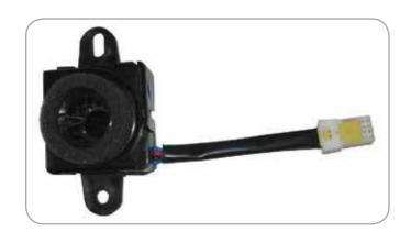
This sensor indicates temperature in the cabin of passenger cars. Since it uses a fan to continuously draw air past the thermistor for an accurate temperature reading, it requires no venturi tube.
