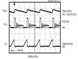
SWITCHING WAVEFORMS (NEGATIVE OUTPUT)
