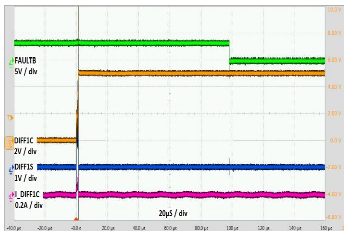
Figure 14. DIFF1C Short to 5V Vbus
