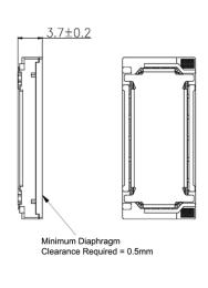
General tolerance = ±0.2 mm and all measurements in mm unless otherwise noted.
