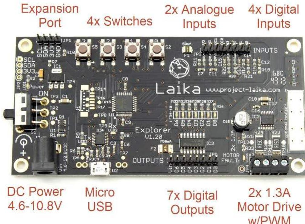
The Laika Explorer board provides powerful robotics control for the Raspberry Pi. Connect with USB and start with Scratch or Python.
