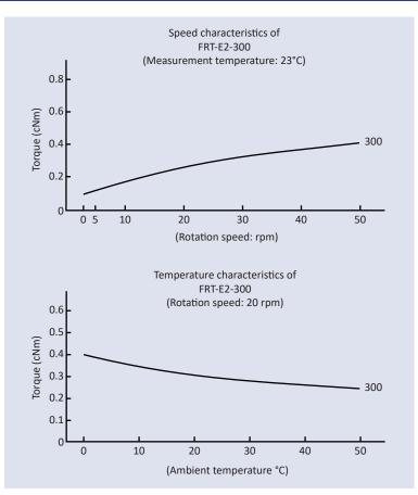
Speed characteristics: A rotary damper's torque varies according to the rotation speed. In general, as shown in the graph to the left, the torque increases as the rotation speed increases, and the torque decreases as the rotation speed decreases. In addition, please note that the starting torque slightly differs from the rated torque.
