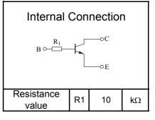
Transistors with Built-in Resistor
