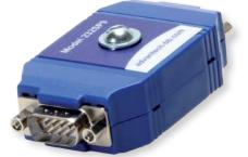
Model 232SP9 protects RS-232 ports from damage caused by large voltage peaks from lightning and other power problems. The surge protector uses 600W Transient Voltage Suppressors to protect all 9 pins. It has one DB9 male and one DB9 female connector with all 9 pins passing straight through. The TVSs are connected between the ground screw and pins 1, 2, 3, 4, 5, 6, 7, 8 and 9. The 232SP9 will suppress any voltage levels above 12 Volts without affecting the normal RS-232 data.
