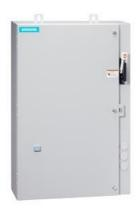
Non-reversing motor starter Size 1 Three phase full voltage Solid-state overload relay OLRelay amp range 10-40a 110-120/220-240VAC 60HZ coil Combination type 30Amp circuit breaker Encl NEMA type 4X 316 S-steel Water/dust tight noncorrosive Extra-wide enclosure
