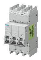
Miniature circuit breaker 240 V 14kA, 3-pole, C, 0.5A, D=70 mm according to UL 489  $\,$
