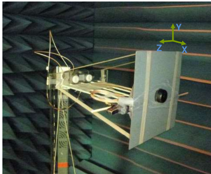
Figure 2. Peak gain, efficiency and radiation pattern measurements.
