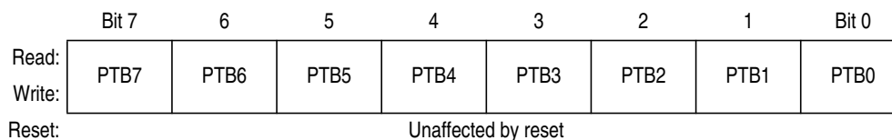
Figure 11-5. Port B Data Register (PTB)
