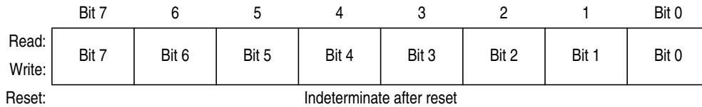
Figure 16-15. TIM1 Channel Register Low (T1CHxL)
