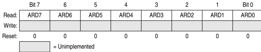
Figure 13-19. ESCI Arbiter Data Register (SCIADAT)
