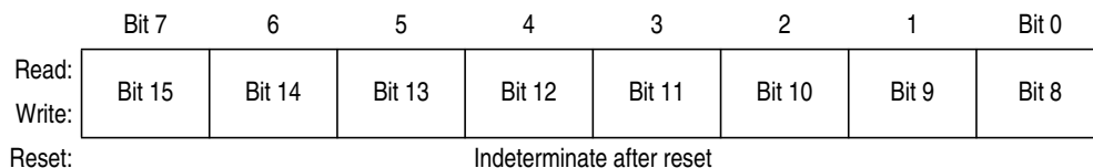
Figure 17-12. TIM2 Channel x Register High (T2CHxH)
