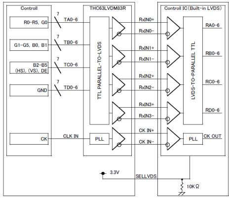
When using "6-bit Transmitter", please connect the unused channel of the control IC receiver as described in the diagram below.
