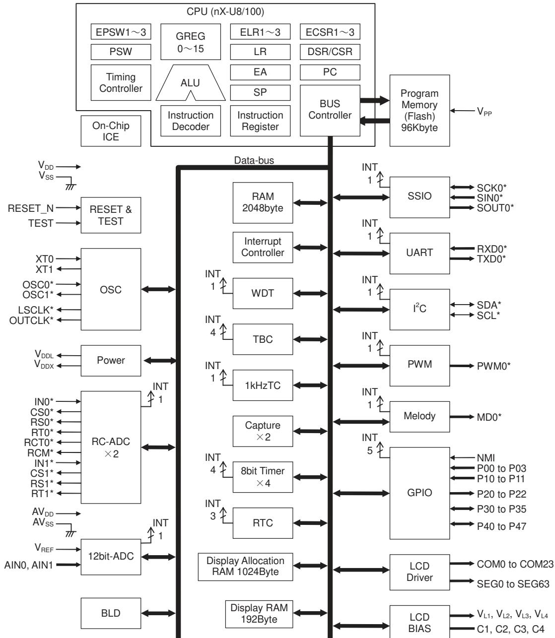
**Figure 2 ML610Q436 Block Diagram**
