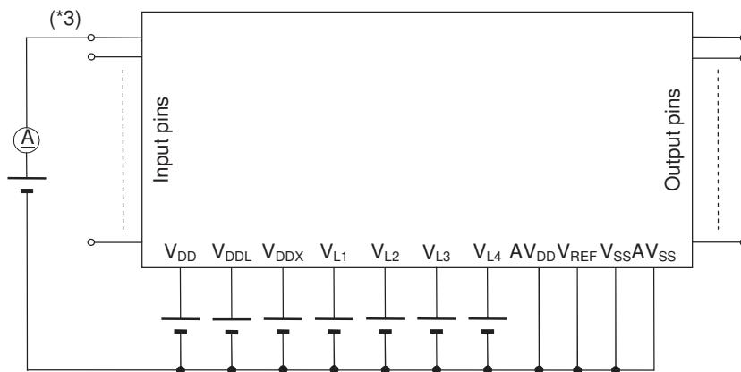
\*3: Measured at the specified output pins.
