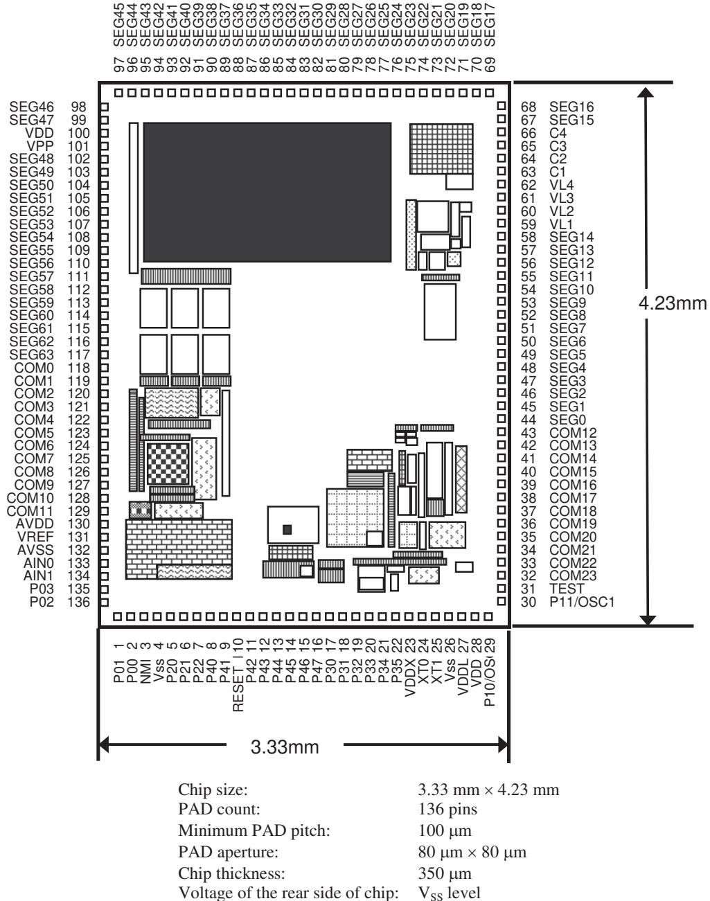
**Figure 6 ML610Q436 Chip Layout & Dimension**
