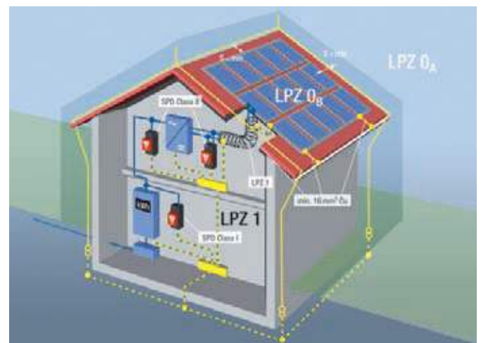
Figure 2: Building installation with external lightning protection system, in compliance with air termination distances
