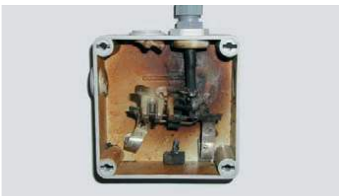
Module box after lightning strike
