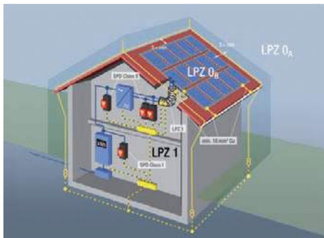
Figure 6: Building installation with external lightning protection, not in compliance with air termination distances
