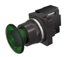
30mm BlackMax, Epoxy Coated Corrosion Resistant Complete Metal Unit Illuminated Push-Pull Operator Full Voltage, 24V AC/DC LED Lamp Mushroom Head Cap Small 1 3/4" (44.5 mm) Plastic, Green 3 Position Pull-Momentary/Push-Maintained UL Listed, CSA Certified NEMA 1,3,3R,4,4X,12,13 & Automotive Standards
