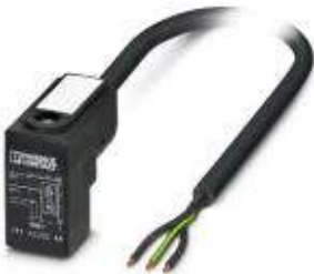
Sensor/Actuator cable, 3-position, PVC, Black RAL 9005, Free cable end, on C valve plug (8 mm), with 1 LED, connected with Z diode, Cable length: 2 m
