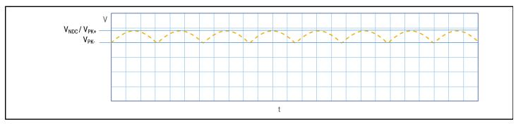
The applied peak-to-peak ripple voltage shall not exceed 0.1 x  $V_{\rm NDC}$ . The peak voltage shall not exceed the rated voltage  $V_{\rm NDC}$ .
