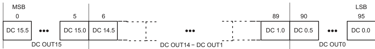
Figure 15. Dot Correction Data Packet Format
