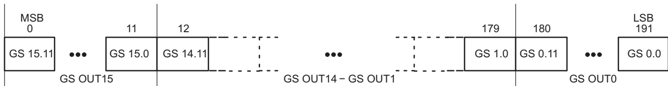
Figure 17. Grayscale Data Packet Format
