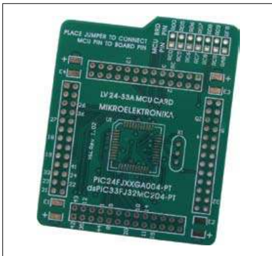
Figure 35: Empty MCU card MCU Card 12
