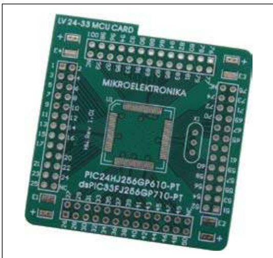
Figure 17: Empty MCU card MCU Card 6
