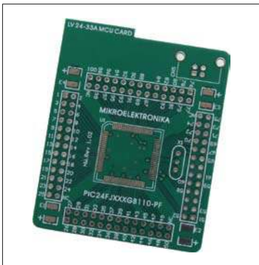
Figure 47: Empty MCU card MCU Card 16
