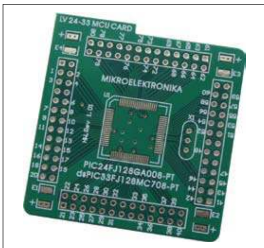
Figure 8: Empty MCU card MCU Card 3
