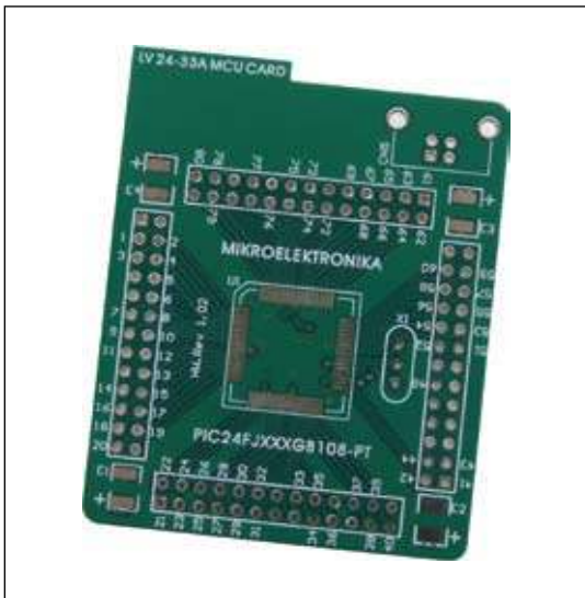
Figure 41: Empty MCU card MCU Card 14
