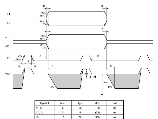
**Remark** The MAX. in the table above shows the operation range in which the output characteristics are kept almost enough for general purpose.
