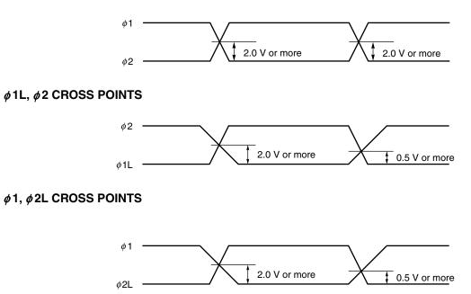
**Remark** Adjust cross points ( $\phi$ 1,  $\phi$ 2), ( $\phi$ 1L,  $\phi$ 2) and ( $\phi$ 1,  $\phi$ 2L) with input resistance of each pin.
