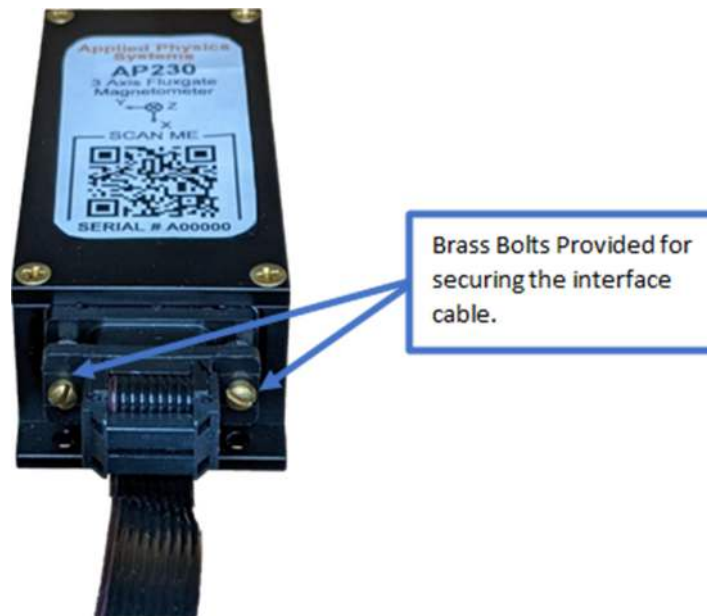
Figure 20 Mounting Sensors and Brass Bolts
