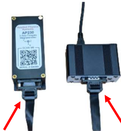
Figure 3 AP230 Connected to Interface Box with the Interface Cable Provided
