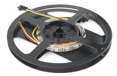
**Description:** These are bare addressable 1 meter long 5V RGB LED strips that come packed with 60 WS2812s per meter. As these are bare LED strips that have no protective coating, your project won't be water proof but there is access to each WS2812 LED and each strip length can be easily modified. You will be able to control each LED RGB individually giving you the ability to create cool lighting effects for your car or perhaps under cabinet lighting in your kitchen!
